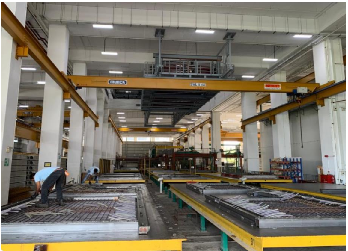
The ICPH produces selected precast components off-site.
