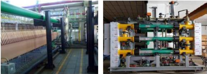
Chemical engineering solutions, including the manufacture of on-site chlorine and sodium hypochlorite generation systems. These help clients reduce dependency on suppliers and lower safety risks from transport and transfer of these chemicals.
